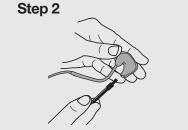
Hold your earphone monitor with the bore holes facing down. Use the cleaner wire to gently scrape any debris from the bore holes.
